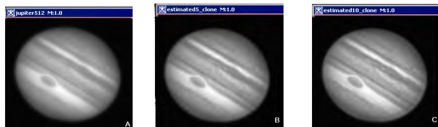
Figure 2. The original image of Jupiter in grayscale (A), the estimate image after five iterations (B), and the final estimate after 10 iterations (C).
