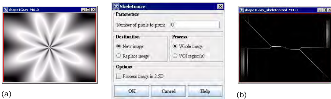
Figure 24. Skeletonize operation: (a) the original image, (b) the result after applying the operation with the parameters shown in the dialog box
