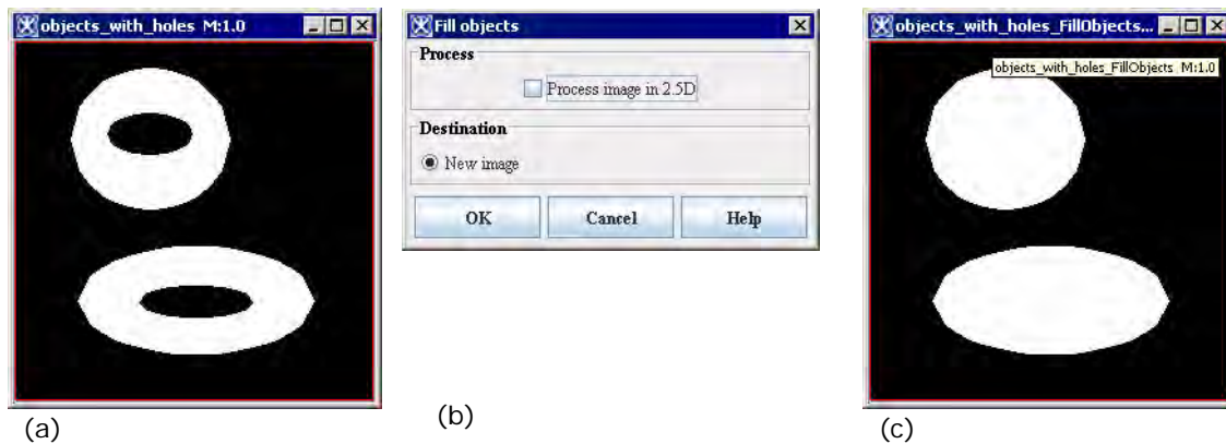
Figure 14. The Fill Holes algorithm: (a) the original image; (b) the Fill Objects dialog box; (c) the result image
